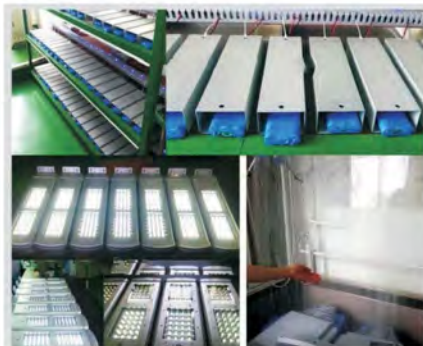
Battery Aging, LED Aging And Waterproof Testing
